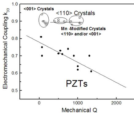
Fig. 5 The relationship between Electromechanical coupling and mechanical Q for crystals and ceramics.
