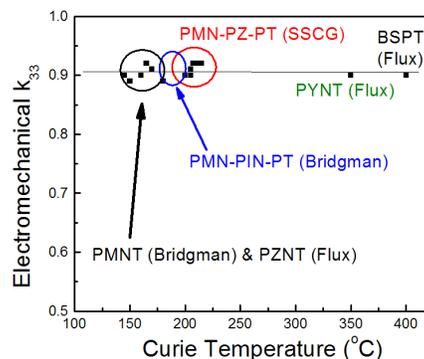
Fig. 1 Electromechanical coupling  $k_{33}$  as function of  $T_C$ .
