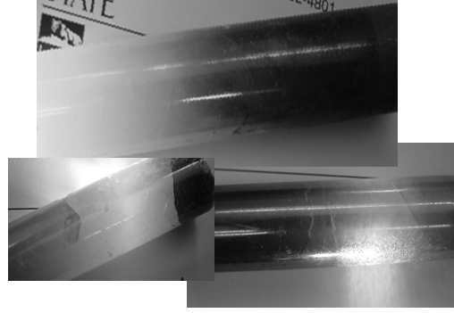
Fig. 5 Photos of the PMNT crystals with different modifications grown using the Bridgman method.
